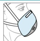
**Ensure** that the face piece collapses slightly under negative pressure that is created with this procedure.
